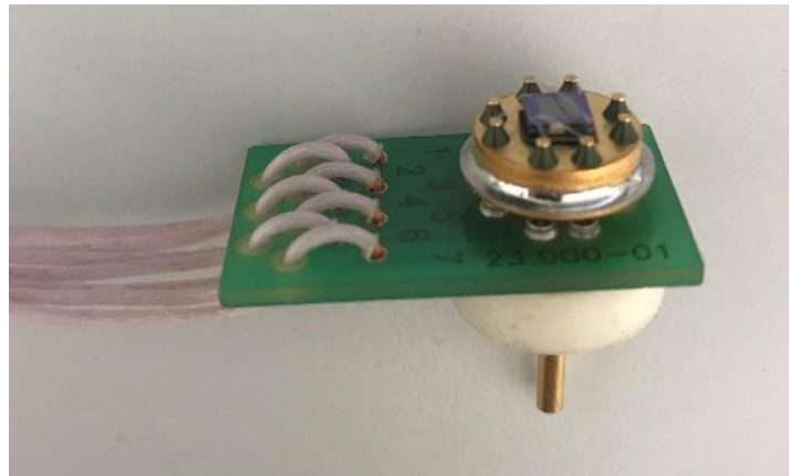
Fig. 5. Assembly of pressure sensor PDA-NFL
