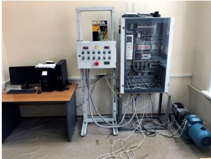
Fig. 4. Laboratory bench for the study of synchronous machines
